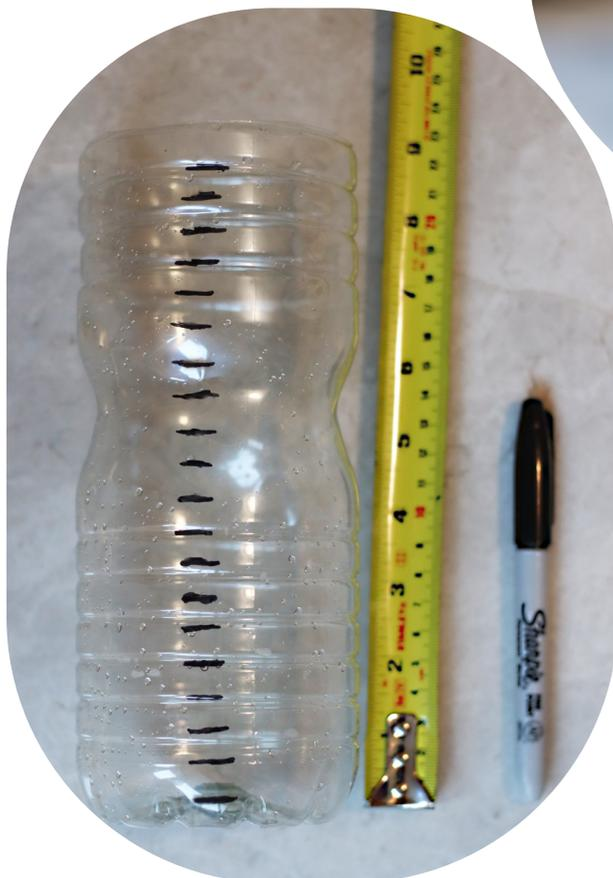
2. Use the ruler or measuring tape to mark measurement lines on the side of the bottle. Start from the bottom and make marks at regular intervals, such as every centimeter or half-inch. Use a permanent marker to make the lines clearly visible.
